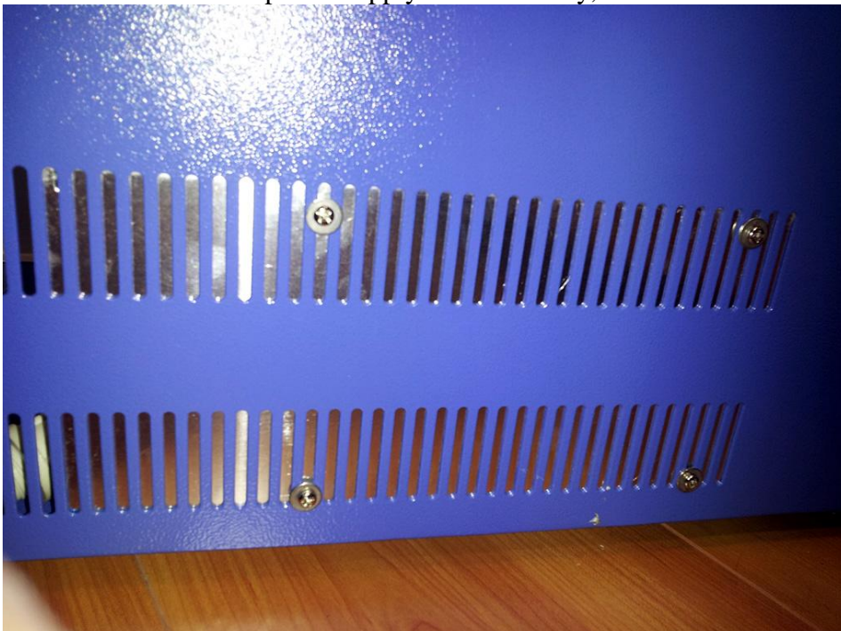
Fig 25. Mounting screws for the DC24V power supply Step 6. Front panel
