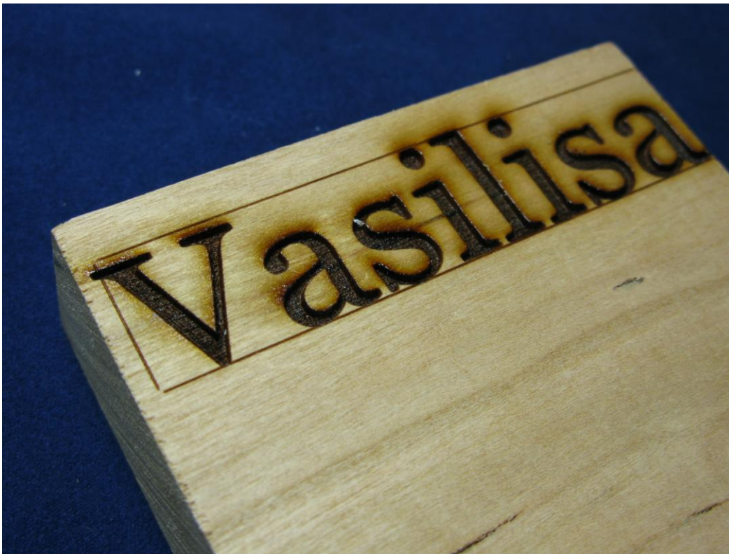
Fig 42. Deep engraving on hardwood (approximately 1.5mm)
